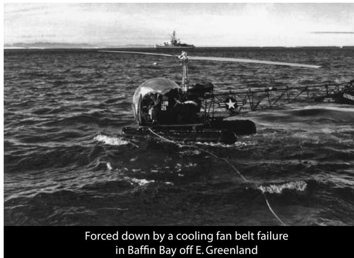
Forced down by a cooling fan belt failure in Baffin Bay off E. Greenland
